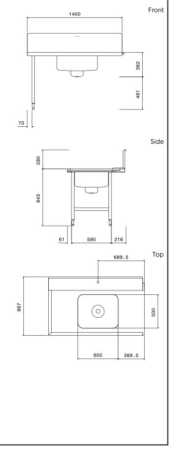
Handling System for Pot & Pans Pre-wash/Unloading Table with Deep Left Basin, 1400mm
